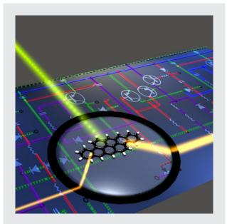
Figure 1: A molecular integrated circuit. An artistic representation of a fully optical circuit created on building bocks such as the single molecule optical transistor. In the black circle, a molecule is amplifying a light signal (yellow), exactly as a transistor does on electronic signals. The control over the amplification is given by a second light beam (green), which decides whatever the molecule is amplifying, attenuating or leaving the input signal unaltered.
