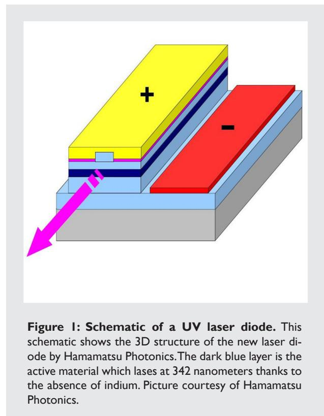
**Figure 1: Schematic of a UV laser diode.** This schematic shows the 3D structure of the new laser diode by Hamamatsu Photonics. The dark blue layer is the active material which lases at 342 nanometers thanks to the absence of indium. Picture courtesy of Hamamatsu Photonics.
