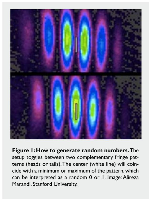
**Figure 1: How to generate random numbers.** The setup toggles between two complementary fringe patterns (heads or tails). The center (white line) will coincide with a minimum or maximum of the pattern, which can be interpreted as a random 0 or 1. Image: Alireza Marandi, Stanford University.
