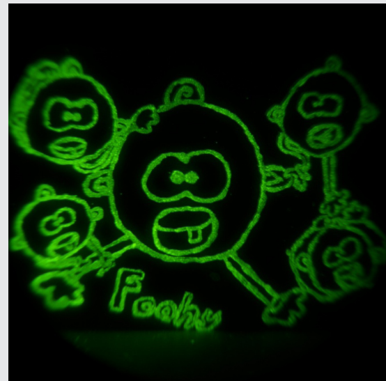
Figure 2: Super glow painting. Five monkeys were drawn using NIR persistent paint that was made by mixing NIR persistent powder into a water-based indoor wall paint. The picture was initially drawn by Grace Pan and traced by Zhengwei Pan. The image was taken using a digital camera with a night vision monocular in a dark room. Credit: Zhengwei Pan and Feng Liu/University of Georgia, USA.
