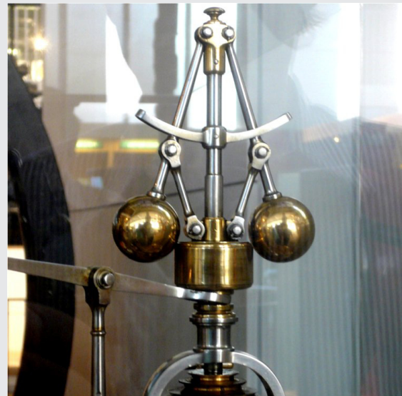
Figure 1: Mechanical automated feedback. James Watt's famous centrifugal governor illustrates the use of an intrinsic classical feedback mechanism to stabilize a system. The heavy balls at the end of the levers are driven away from the rotational axis as the rotational speed increases. This increases the rotational energy of this device, and stabilizes the angular speed of the machine, which drives the centrifugal governor. Picture: Mirko Junge, Science Museum London.
