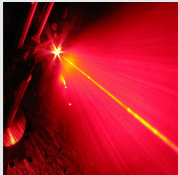
**Figure 1: A random laser flash of light.** A random laser (red) shines light in all directions while it is pumped by a standard unidirectional laser (yellow).
